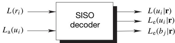
Figure 4.11: Soft-in/soft-out decoder
